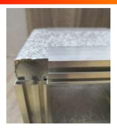
For length assembly of the ventilation channels, the common profiles used are the I-profiles together with H-profiles. By sliding the H-profile into the I-profile an invisible connection can be achieved. The 90° degree corner pieces are place underneath the I-profile at the corner, see photo left.
